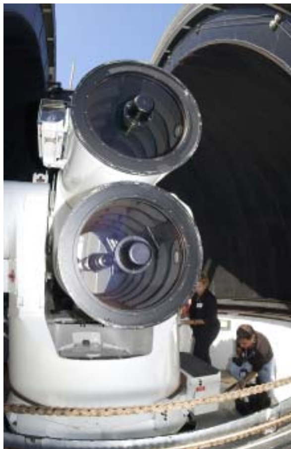
This long-range tracking telescope on Playalinda Beach, north of KSC, uses two lenses: on top, a 400-inch lens for 35mm film, and on the bottom, a 200-inch lens for video.
