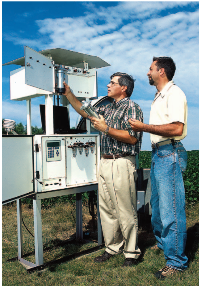
Laboratory director Jerry Hatfield and technician Kenwood Scoggin examine a particulate sampler during air quality studies in Iowa.
