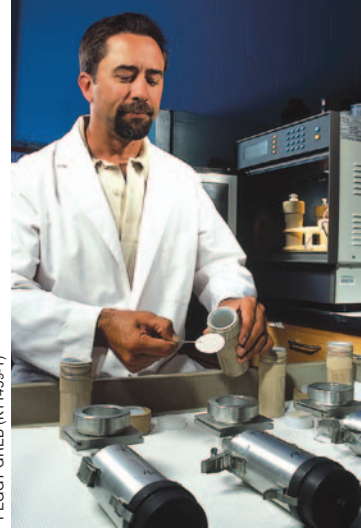
Technician Kenwood Scoggin prepares particulate-filter samples for microwave-assisted extraction as part of the liquid chromatography/mass spectrometer process to identify materials attached to particulates collected in rural Iowa.
