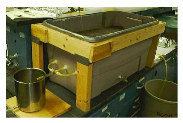
Figure 4. Pilot-Scale Bioretention Setup
