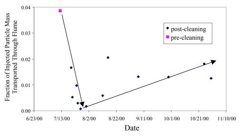
Figure 3: Change in suspended sediment transport over time observed in 2000. Arrows indicate two major trends. Deposition increased (and particle throughput decreased) initially after the beds were cleaned. Deposition continued to increase for two weeks after cleanout. Later, additional particle throughput occurred as the bed became plugged with deposited silts.
