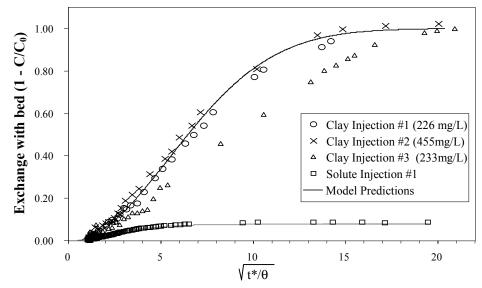
Figure 5: Modeling of results from Figure 4. Fundamental models for stream-subsurface exchange of solutes and colloids successfully predicted the observed exchanges until clay deposition became sufficient to violate the assumption of a clean bed. t\* is a dimensionless time based on a bedform length scale and characteristic pore water velocity;  $\theta$  is the porosity of the bed sediment.
