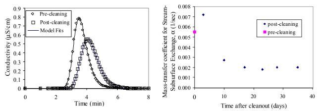
Figure 2. Left Panel: Curves of solute concentration vs. time measured at downstream end of flume following pulse inputs at the upstream end, before and after cleaning of the gravel bed. Additional tailing of the pulse shows that removal of silts from the bed increased stream-subsurface exchange. Right Panel: Following cleaning of the bed, exchange decreased considerably due to ongoing siltation.
