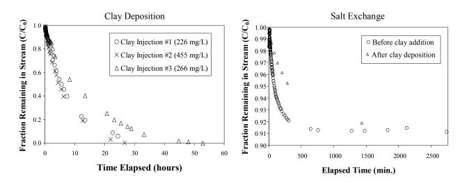
Figure 4: Clay deposition and solute exchange measured in a laboratory flume with a sand bed. Accumulation of clay reduced the rate of stream-subsurface exchange and hindered subsequent clay deposition. Note *extreme* difference in scale between the two figures.
