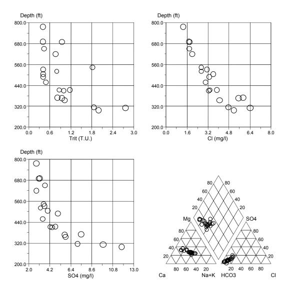
**Figure 3.** Plots of tritium and dissolved constituents versus depth and Piper plot for production wells in the Sheahan well field and University of Memphis well sampled in 1999.
