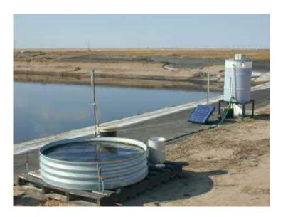
Figure 2. Photograph of the evaporation pan system in the field.
