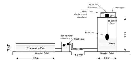
Figure 1. Diagram of the portable Class-A pan system for use at lagoons.
