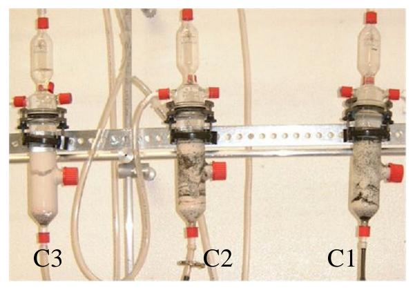
**Figure 1.** 0.5-L laboratory-scale anaerobic columns used to investigate the microbial mobilization and biotransformation of arsenate sorbed onto activated alumina under simulated landfill conditions. **(C1)** Biological column fed a synthetic landfill leachate containing both inorganic and organic components. **(C2)** Control column fed with an inorganic leachate (lacking organic substrates). **(C3)** Abiotic column fed with an inorganic leachate
