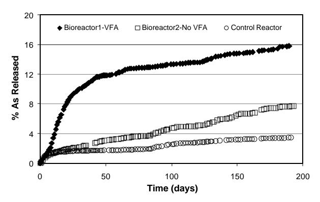
**Figure 4.** Release of arsenic (As) from activated alumina with sorbed arsenate in anaerobic columns percolated with model landfill leachate. Bioreactor 1 and 2 were inoculated with anaerobic sludge, but only bioreactor 1 was supplied with organic substrate, volatile fatty acid mixture (VFA). The control reactor was not inoculated.
