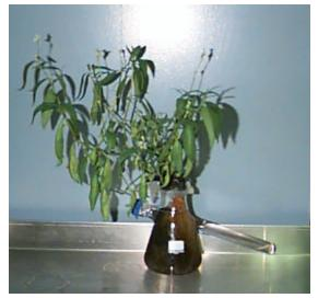
Figure 2. Experimental system used to quantify  $O_2$  released from wetland plant roots (*P. pennsylvanicm* shown).
