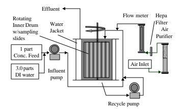
Figure 1. Experimental flow chart of biofilm reactor.
