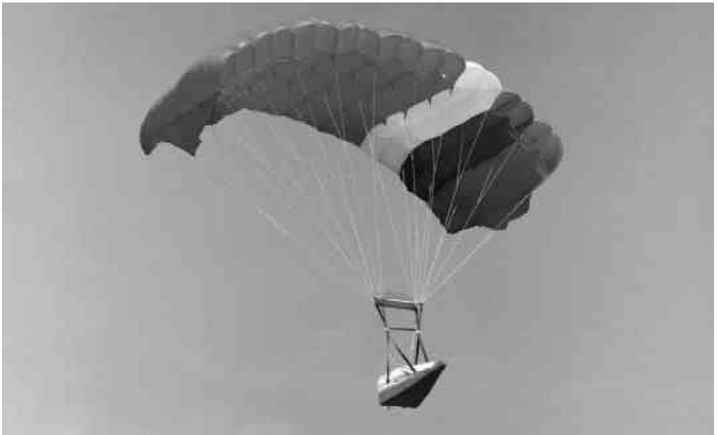
Spacewedge vehicle descending with 288 sq. foot parafoil. NASA photo EC 92-04271-4
