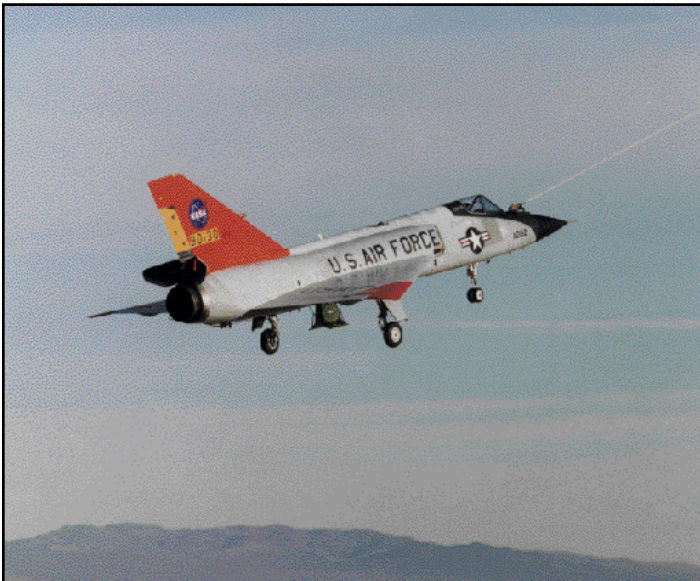
Eclipse project's EXD-01 lifts off under tow by a USAF C-141A aircraft. NASA photo EC97 44357-10
