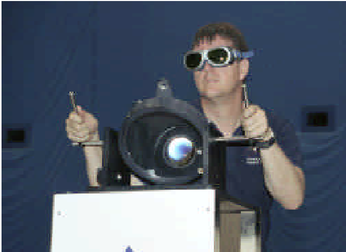
NASA Dryden's Dave Bushman aims the optics of a laser device at a panel of solar cells during the first flight demonstration of an aircraft powered by laser light.
