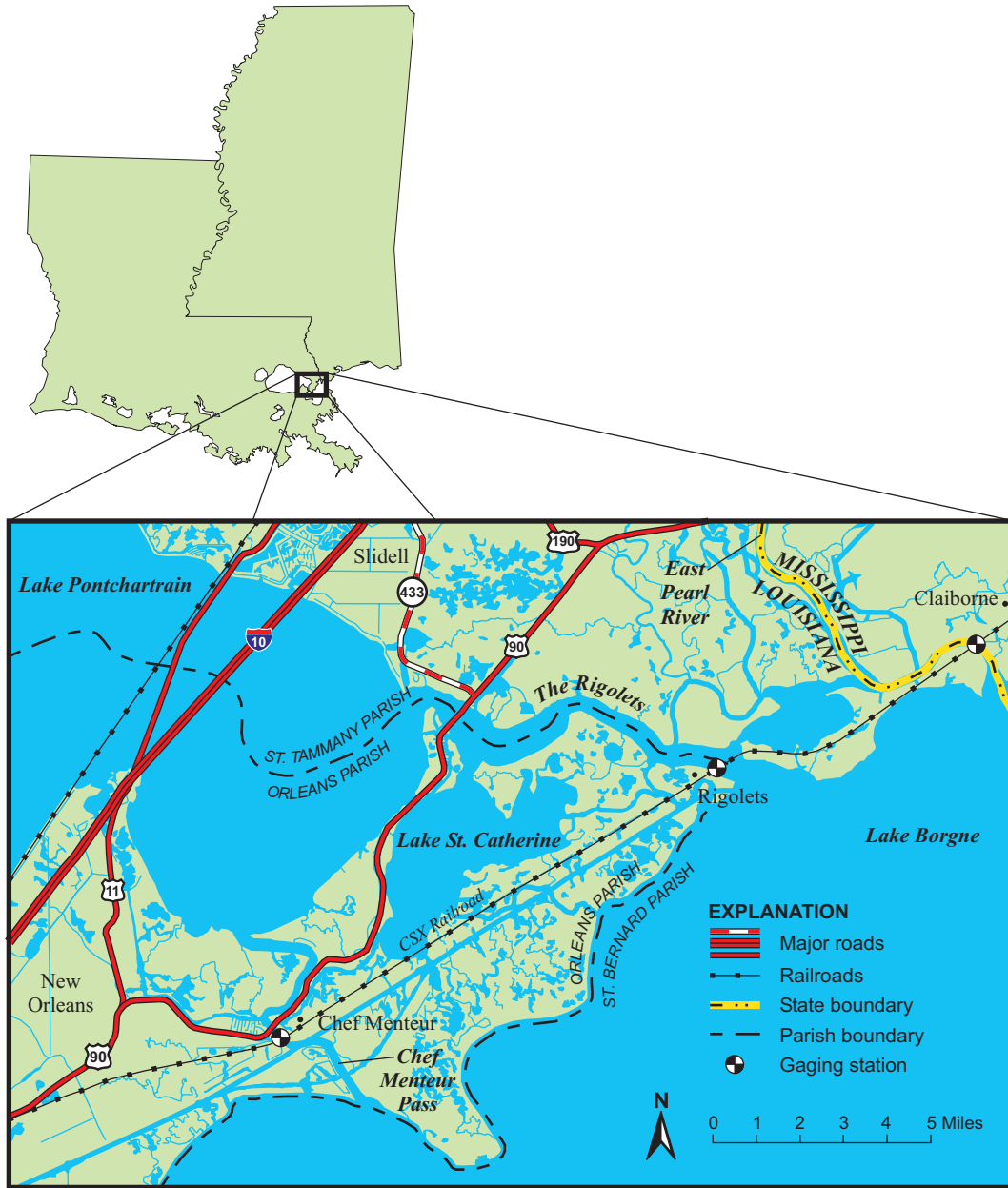
Figure 1. Location of three continuous recording stage, velocity, and water-quality parameter streamgages in the lower Pearl River and Lake Pontchartrain estuaries in Mississippi and Louisiana.
