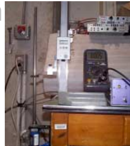
Calibration of Reference Temposonic
