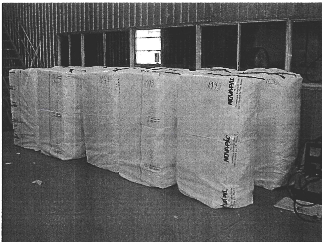
Figure 6. Bales for Study 3 stored near the instrument room in Building 21. Eleven bales were stored in fully coated, woven polypropylene bags.
