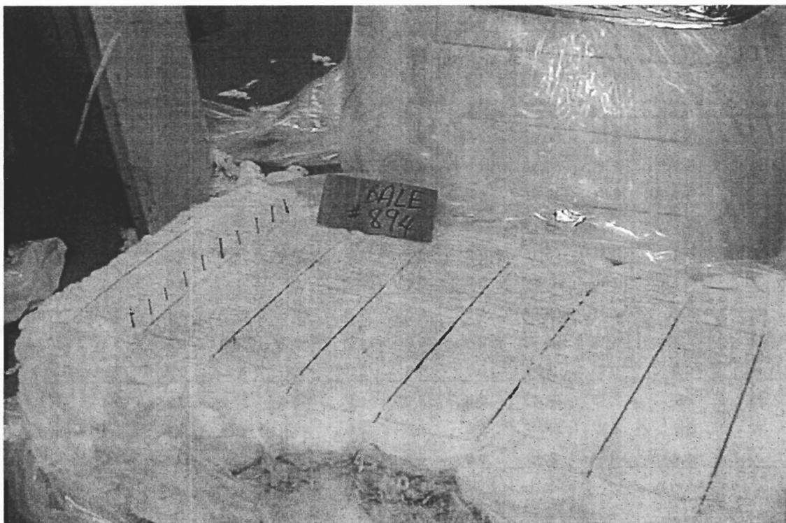
Figure 2. Typical bale divided into 10 layers about 6.4 cm (2.5-inches) apart before sampling.
