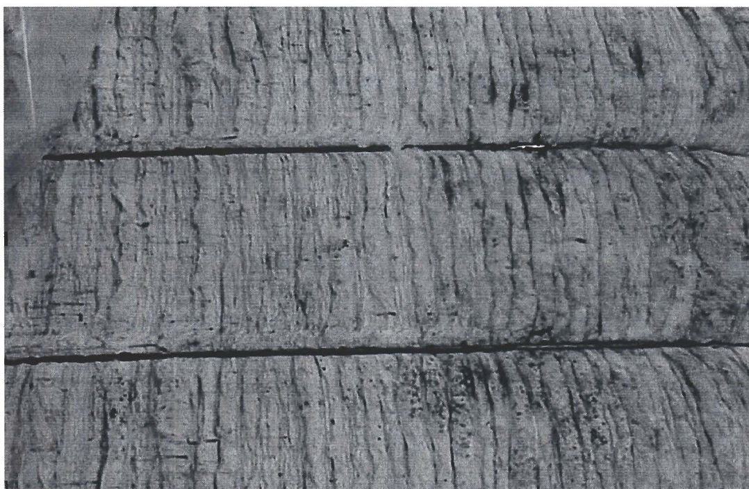
Figure 1. Water damage observed when polyethylene bags were removed after storage.
