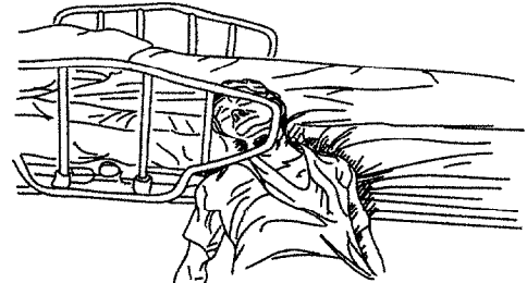
Zone 6 – Entrapment between the rail end and edge of head/foot board
