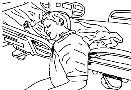
Zone 7 – Entrapment between head or foot board and mattress
