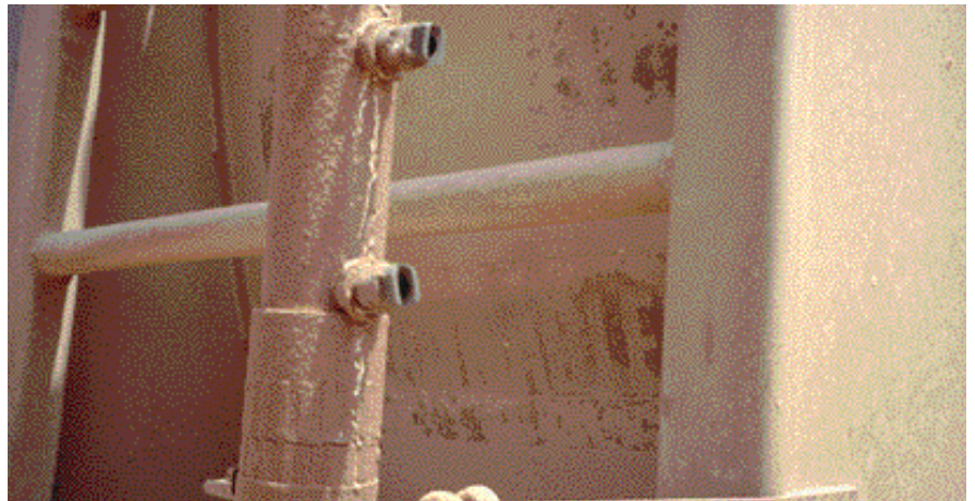
Example of a good piece of application equipment. This truck has a pressurized spray bar with a computerized application system that meters the liquid Chloride with extreme accuracy.
