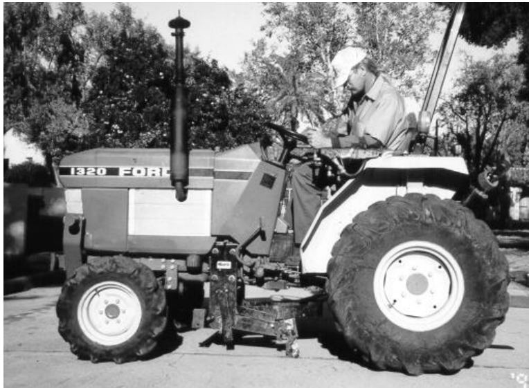
Figure 6. Undercarriage-mounted joint plow.
