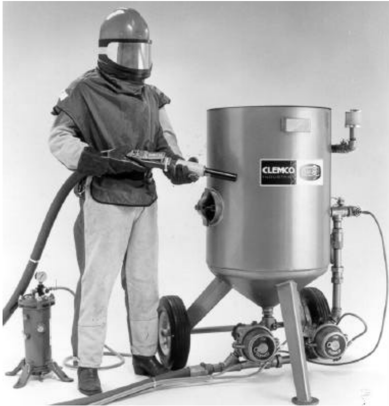
Figure 8. Abrasive blasting equipment.
