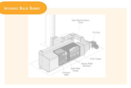
Controlled flame shape of the RSB leads to compact integrated boiler burner designs and more rapid cooling of combustion products.
