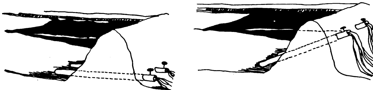
Figures 8-13 and 8-14: Earthen Dams, Cross Sections. Left: Multiple pipes near the bottom with valves to control the flow and retained depth of the water. Right: Pipes installed on an incline to control water depth. The top of the incline determines the height of the retained water and oil.
