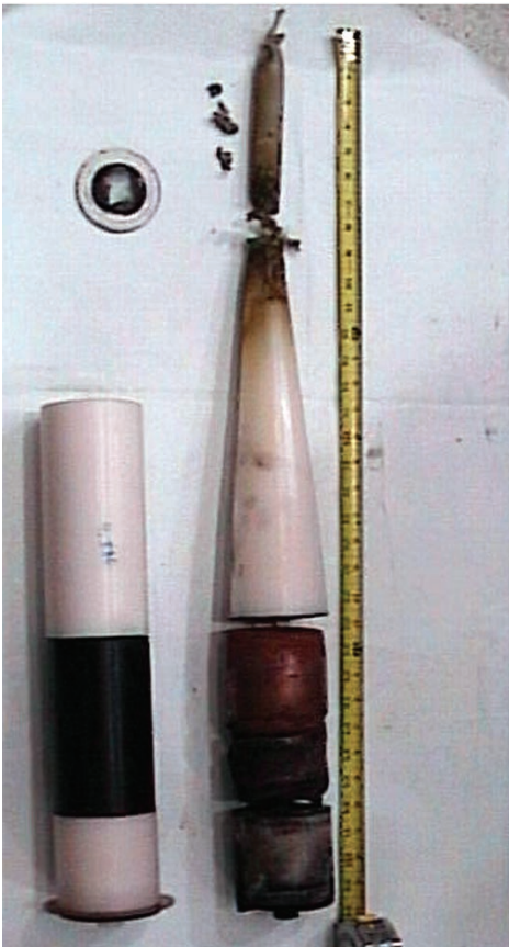
An extrudable piston is shown before and after firing. The piston compresses hydrogen gas in the first stage of the two-stage gas gun.
