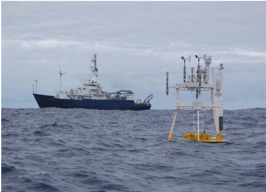
Figure 5. A surface buoy instrumented for surface meteorology, moored off northern Chile since October 2000. Research ships service the mooring once a year; the Scripps Institution of Oceanography's RV Roger Revelle is shown here.
