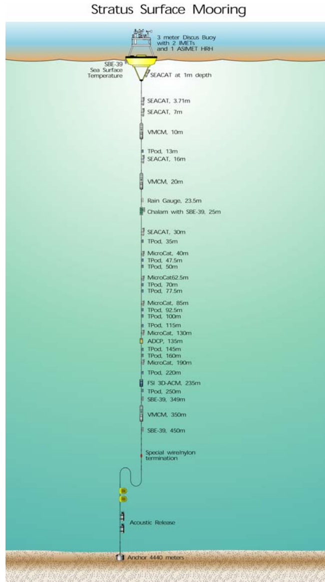
Figure 6. Schematic diagram of the surface mooring deployed by the Woods Hole Oceanographic Institution off northern Chile since October 2000 with support from the NOAA Office of Global Programs and Climate Observation Program. The surface buoy is instrumented to measure surface meteorology. Along the mooring line, SEACAT's measure salinity and temperature; VMCM's measure temperature and velocity of the water, the rain gauge from Dr. Jeff Nystuen of the Applied Physics Laboratory of the University of Washington measures the noise created by raindrops, Tpod's and SBE-39's measure temperature, MicroCat's measure salinity and temperature, and the ADCP or Acoustic Doppler Current Profiler measures ocean velocity as does the FSI 3D-ACM.
