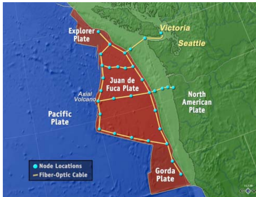
Figure 13. Location and basic structure of the regional cabled observatory proposed for the Juan de Fuca Plate. Canada has become implementation of its contribution, and the U.S. component is proposed as an element of the NSF OOI.
