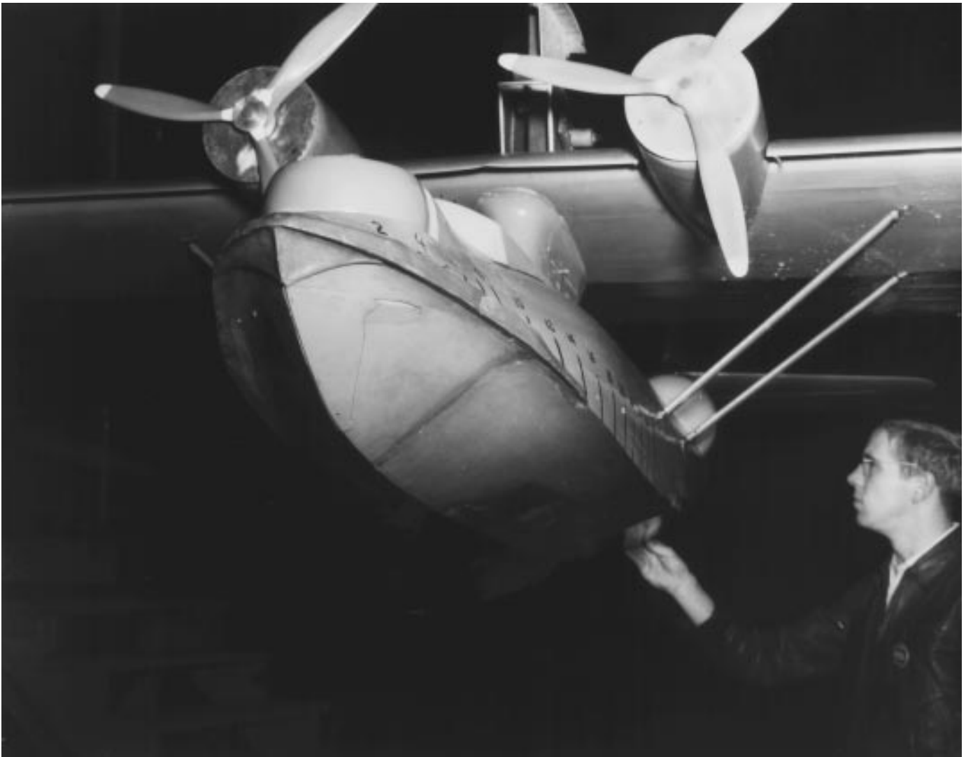
A model of the Consolidated PBY Catalina flying-boat is prepared for tests in the NACA Langley hydrodynamic facilities.
