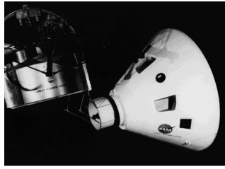
Langley's Rendezvous and Docking Simulator was used by NASA scientists to study the complex task of docking the Lunar Module with the Command Module in lunar
