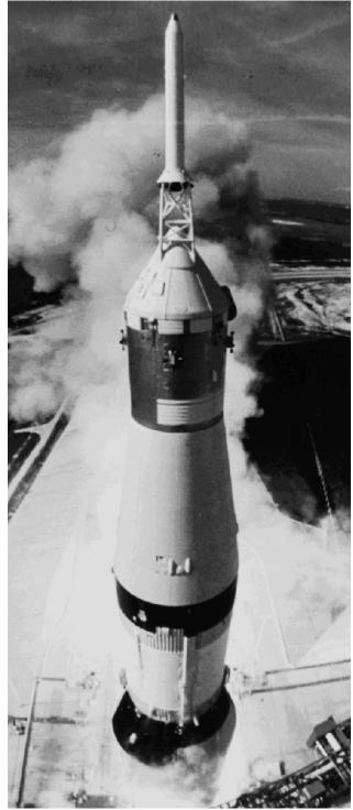
Apollo 11 rises past the launch tower at Pad 39A to begin man's first lunar landing mission. Liftoff occurred at 9:32 a.m., July 16, 1969. The launch vehicle was a Saturn V, developed for the Apollo lunar missions. With the Apollo spacecraft, the Saturn V stood 363 feet tall. Space Shuttle missions are still launched from venerable Pad 39A.
