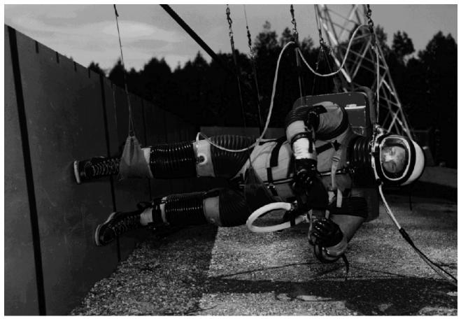
Researchers at Langley Research Center studied astronauts' ability to walk, jump and run using this ingenious lunargravity simulator. The astronauts wore pressure suits that were supported by a system of slings, cables and a trolley that was controlled by the subjects as they performed maneuvers. The facility also studied astronaut fatigue limit and energy expenditure in the one-sixth Earth-gravity conditions.
