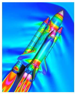
A computer-generated image of the space shuttle showing varying pressures in the airflow
