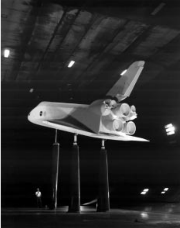
A scale model of the Shuttle Orbiter is mounted inside the 40- by 80-foot test section of a wind tunnel at NASA's Ames Research Center. Instrumented supports provide data on the model's aerodynamic characteristics.
