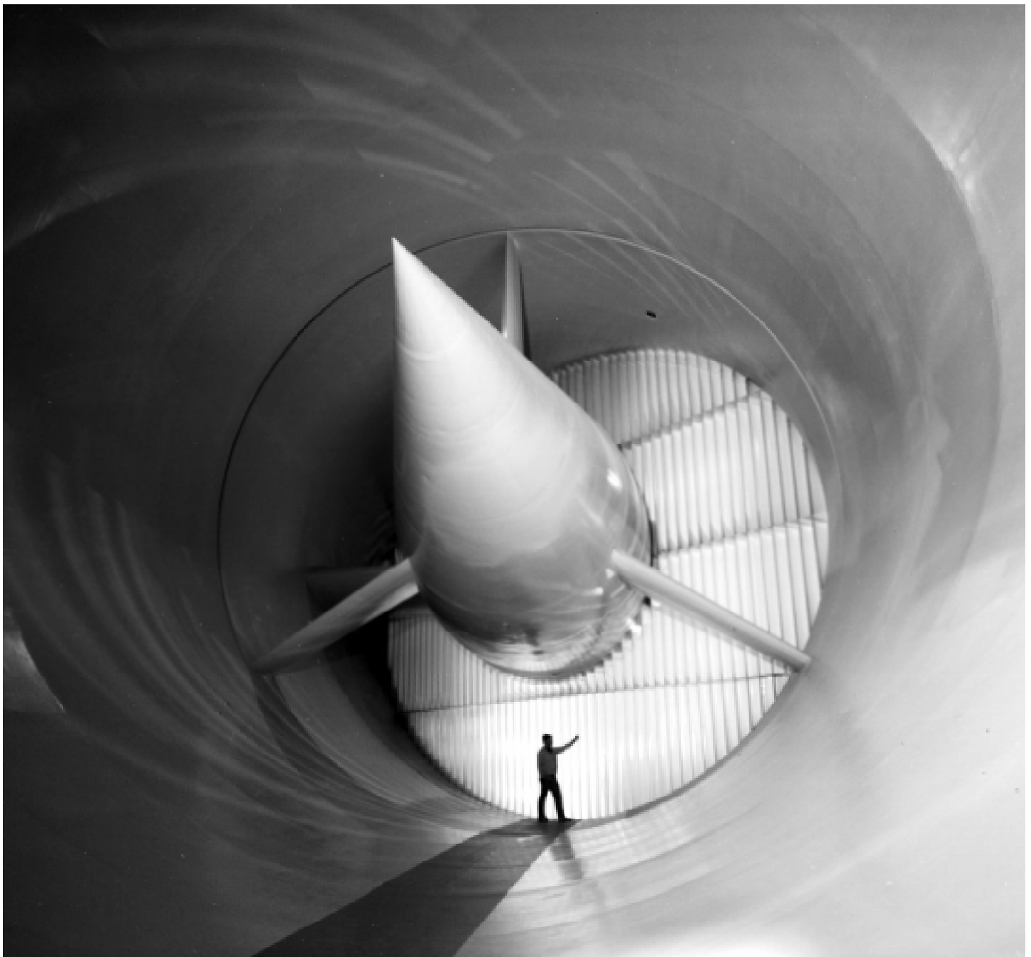
Giant vanes help air flow around a corner in this transonic wind tunnel at NASA's Langley Research Center.
