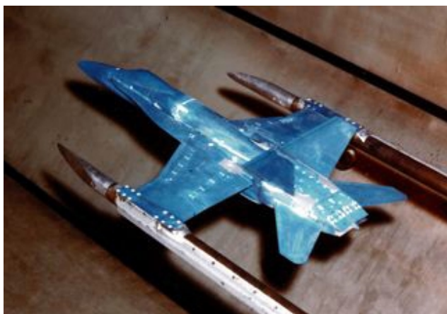
F/A-18 model with 2-D convergent-divergent (CD) nozzles tested in Langley 16-Foot Transonic Tunnel.
