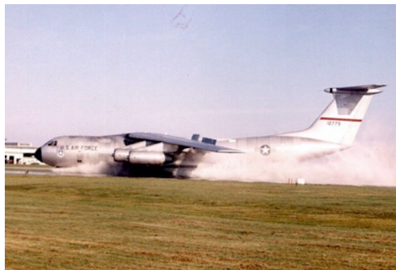
C-141 braking tests in a joint NASA, Air Force, and FAA program at Wallops Flight Facility.
