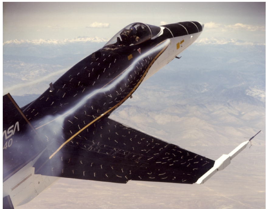
F-18 HARV during flow visualization studies using smoke ejected at apex of LEX and wool tufts on upper surfaces.
