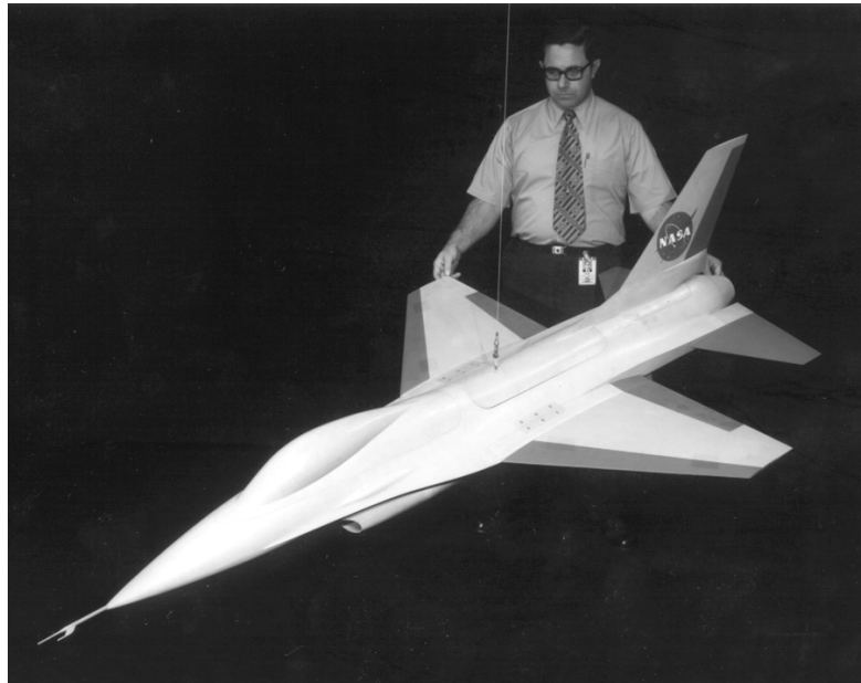
Researcher William A. Newsom, Jr. with the free-flight model of the YF-16 used in tests in the Full-Scale Tunnel.
