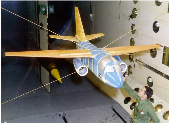
S-3 flutter model in the Langley 16-Foot Transonic Dynamics Tunnel.
