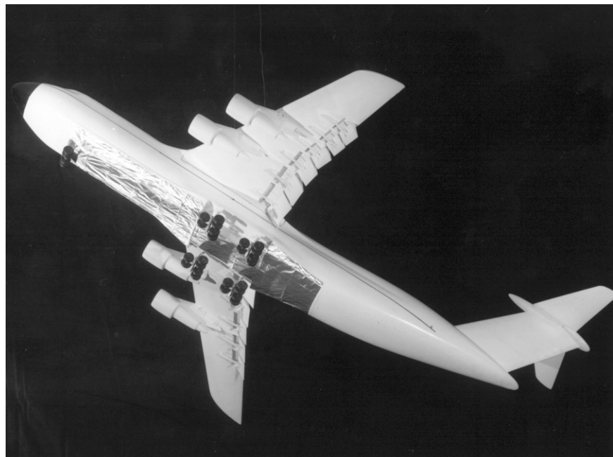
C-5 ditching model with simulated structural skin on bottom of model.
