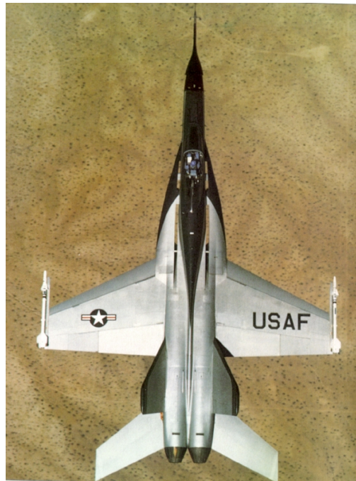
A YF-17 prototype in flight with the open slots in the LEX adjacent to the fuselage.
