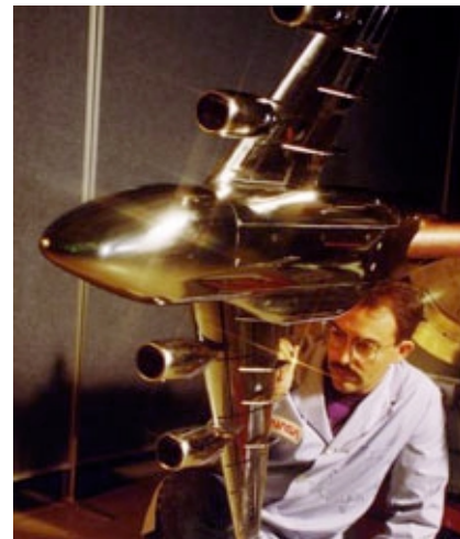
C-17 model mounted in the National Transonic Facility at Langley for aerodynamic studies.
