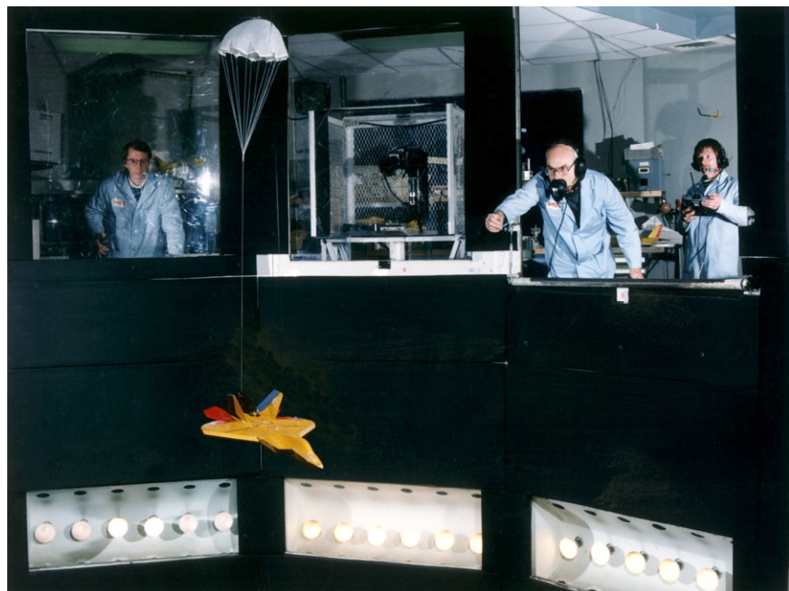
F-22 model during tests in the Langley Spin Tunnel to determine the size of emergency parachute required for spin recovery.
