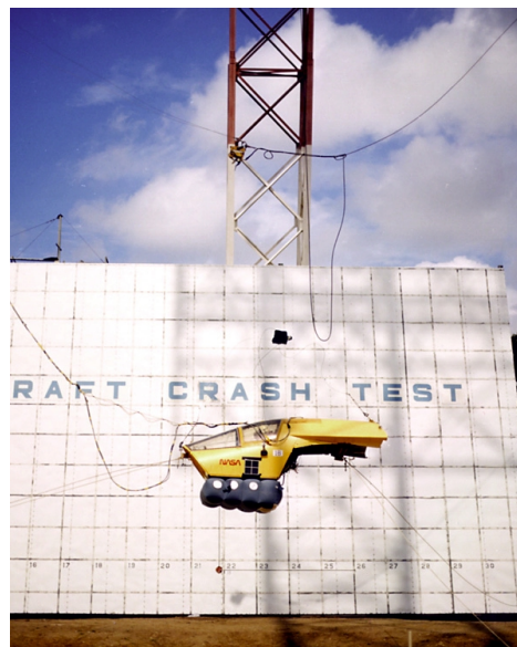
F-111 crew escape module during tests at the Langley Impact Dynamics Research Facility.
