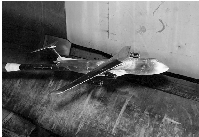
C-5 model mounted for tunnel test section study in the Langley 16-Foot Transonic Tunnel.
