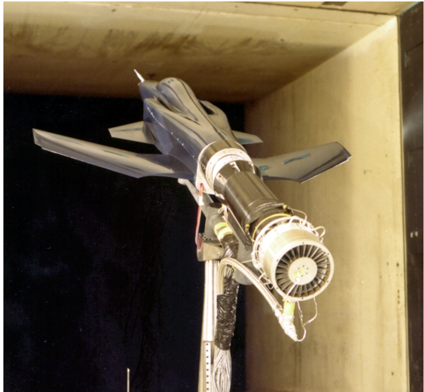
X-29 powered-inlet model tests in the Langley 14- by 22-Foot Subsonic Tunnel.
