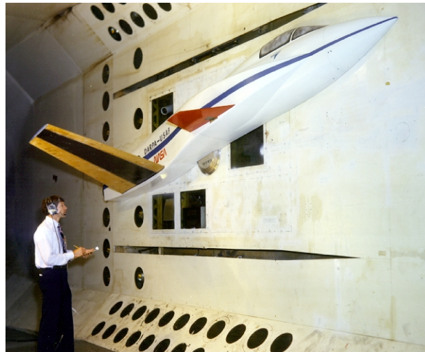
Rodney Ricketts with the Grumman FSW model during aeroelastic divergence tests in the Langley 16-Foot Transonic Dynamics Tunnel.
