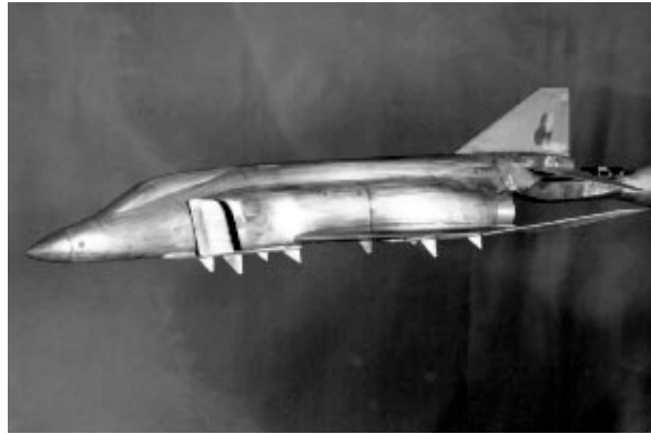
F4H model after modifications with dihedral in outer wings and increased vertical tail.
