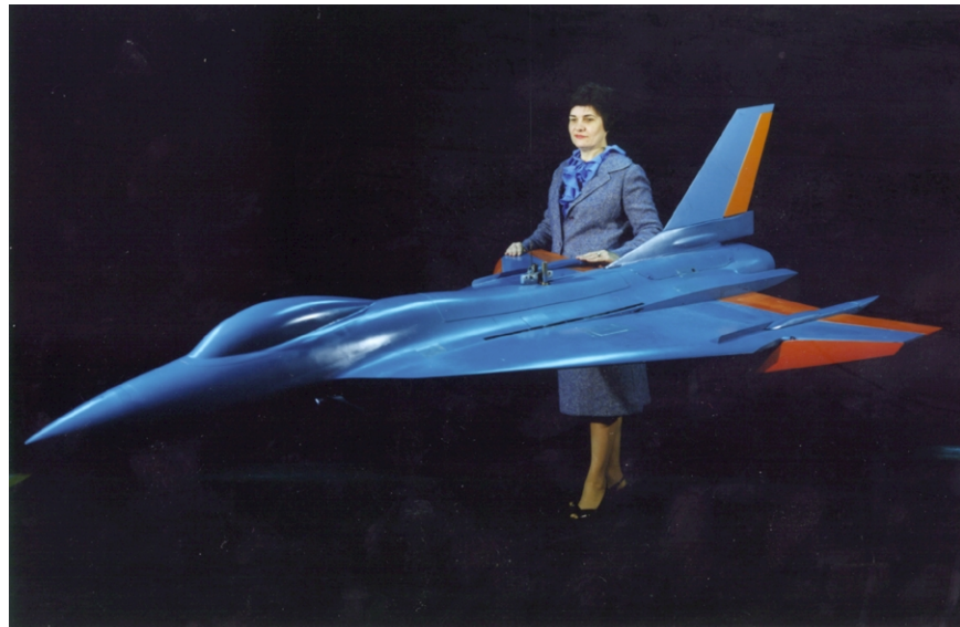
Project engineer Sue B. Grafton with the free-flight model of the F-16XL.
