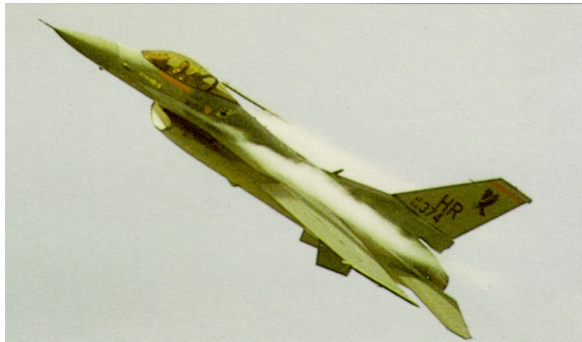
F-16 in a hard turn with wing leading-edge flaps deflected and vortices produced by the sharp wing-body strakes illustrated by condensation.
