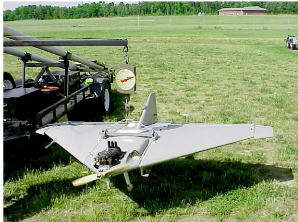
An Exdrone undergoes weight and balance tests.
