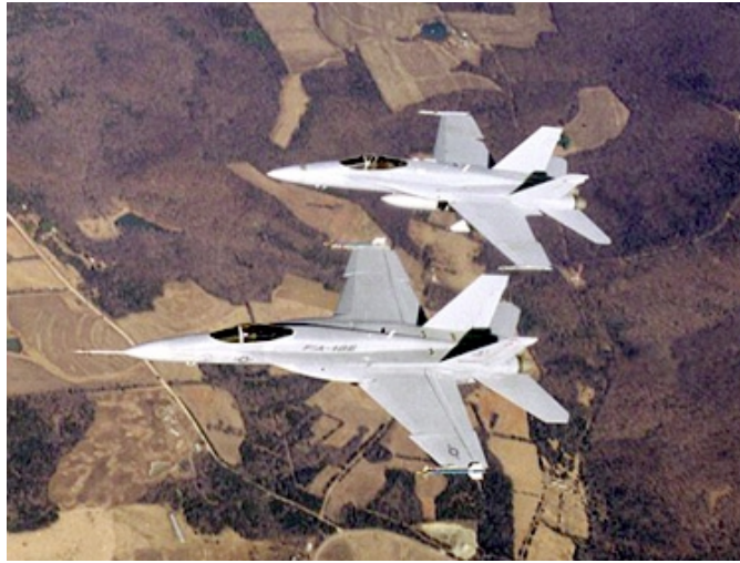
F/A-18E/F (foreground) with redesigned LEX in flight with F/A-18C chase aircraft.
