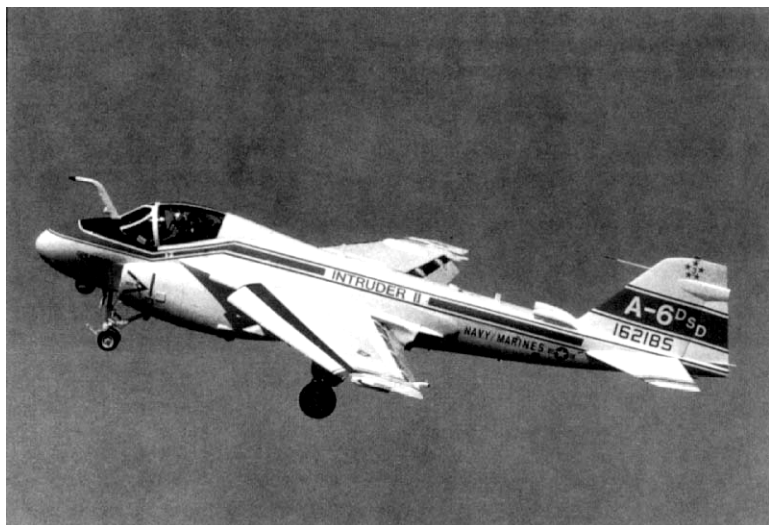
A-6F prototype with aft-fuselage scoops.
