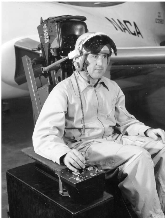
Langley test pilot William L. Alford checks out the side-stick controller in 1954 studies.
