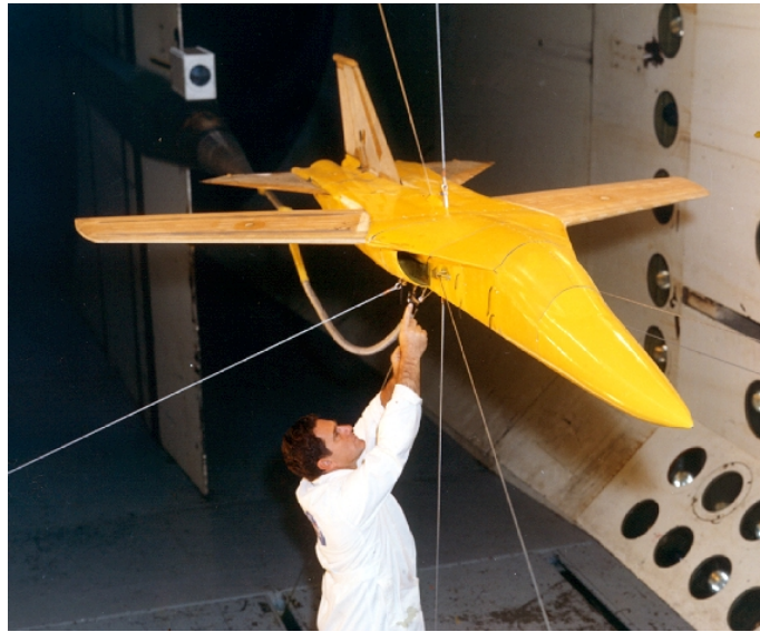
F-111 TACT model mounted for flutter tests in the Langley 16-Foot Transonic Dynamics Tunnel in 1971.
