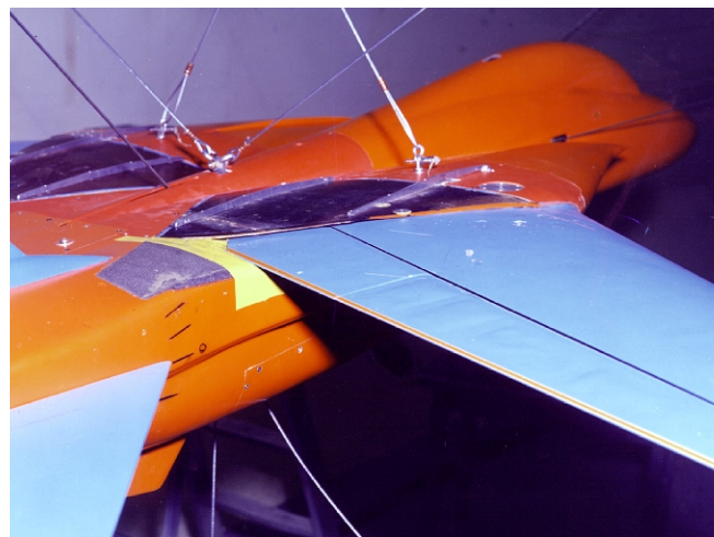
Close-up view of the external over wing cover strakes added to prevent panel flutter.
