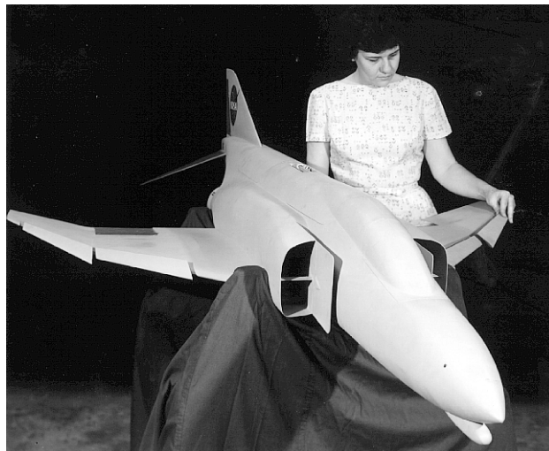
Researcher Sue Grafton with the slatted F-4E model used for free-flight tests in the Langley Full-Scale Tunnel.
