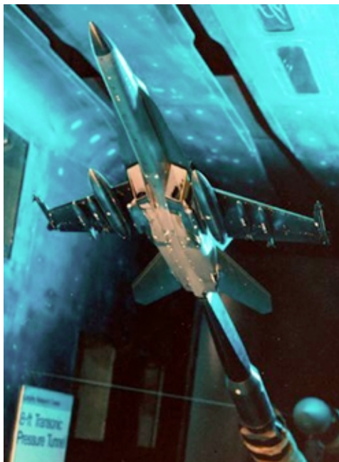
F/A-18E/F model in 8-Foot Transonic Pressure Tunnel for evaluations of the LEX spoiler concept.
