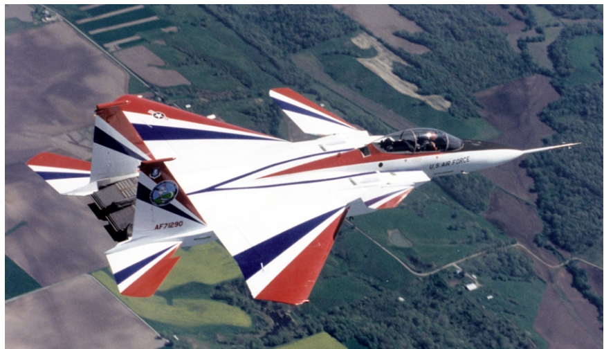
The F-15 STOL/MTD flying with canards and thrust-vectoring nozzles.
