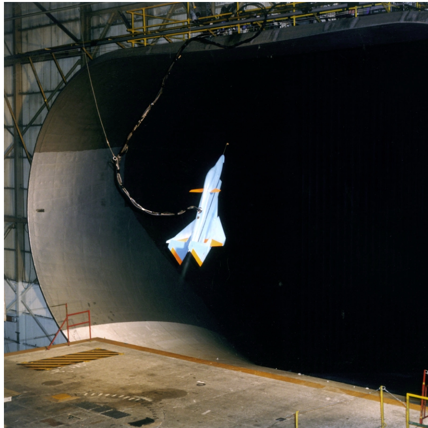
Modified SNAKE model flying at extreme angle of attack using thrust vectoring in the Langley Full-Scale Tunnel.
