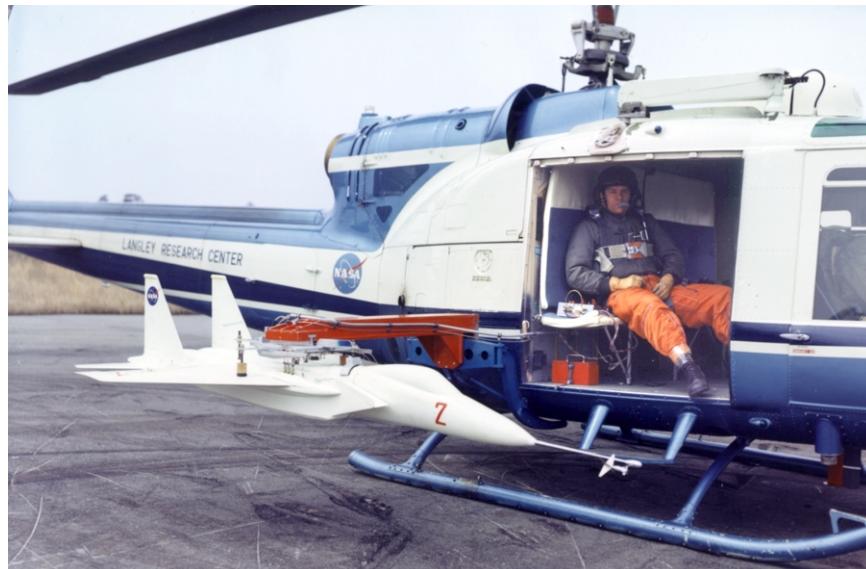
Langley technician Ronald White with one of two F-15 drop models used for research on spin-entry characteristics.
