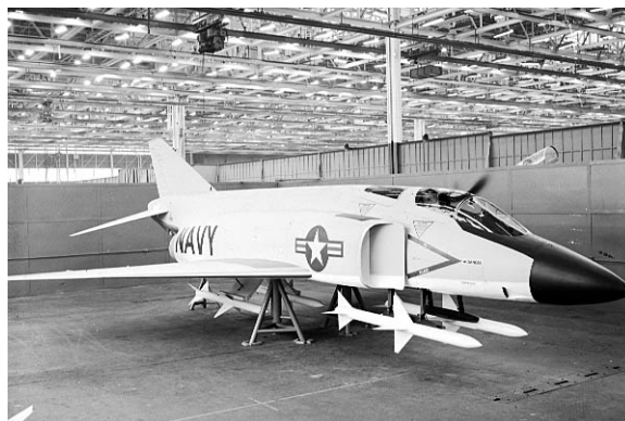
Engineering mock-up of the original F4H Phantom without dihedral in outer wings and 15-deg droop of the horizontal tail.
