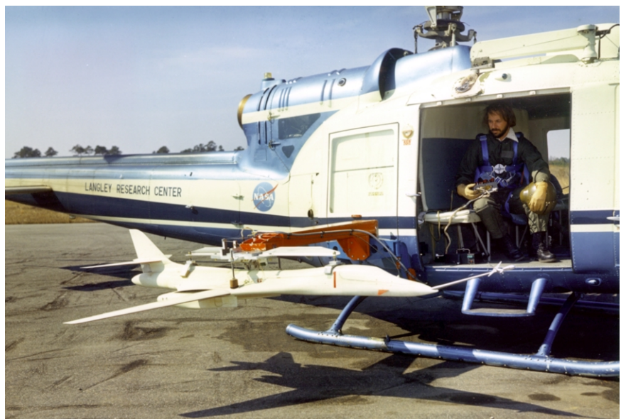
B-1A drop model being prepared for helicopter drop test in 1974.
