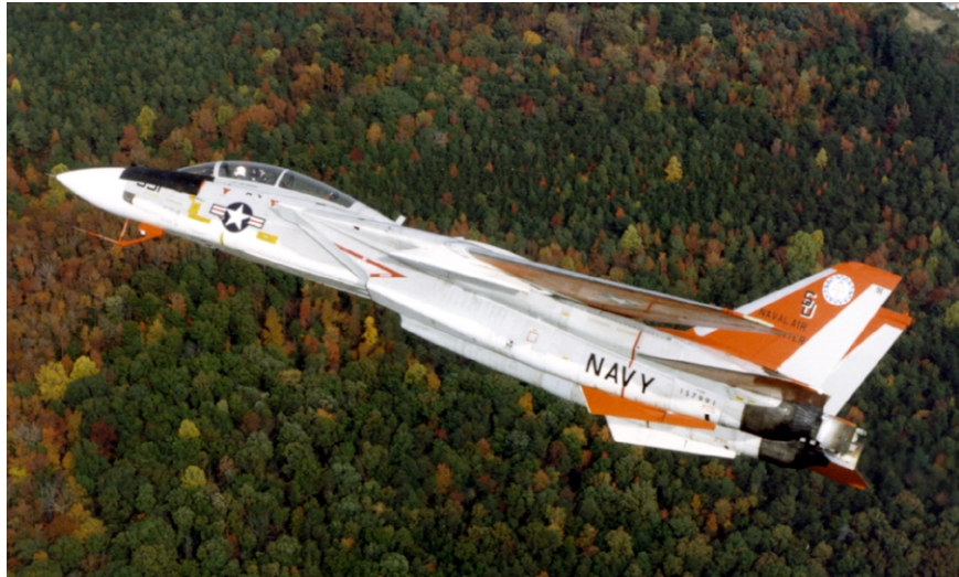
F-14 with experimental yaw vanes in flight over Patuxent River Naval Air Station.
