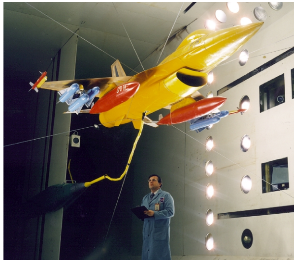
Jerome T. Foughner checks out the F-16 model with external stores mounted in the 16-Foot Transonic Dynamics Tunnel for flutter tests.
