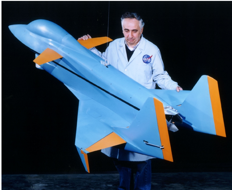
The original Rockwell SNAKE configuration with downturned wingtips and thrust vectoring paddles.
