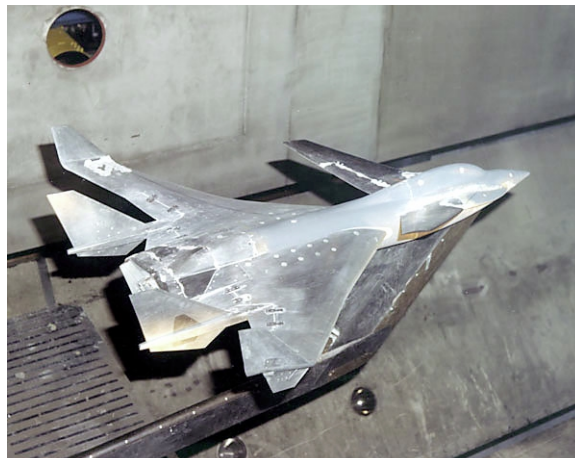
The original HiMAT model with the thrust-vectoring, wedge nozzle in the Langley 16-Foot Tunnel.
