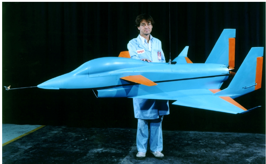
The modified SNAKE configuration after the Langley tests with upturned wingtips, wing leading-edge flaps, enlarged vertical tails, enlarged wing-fuselage strake, and nose strakes.
