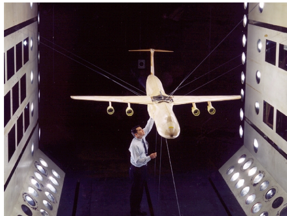
Full-span model of the C-5 in the Langley 16-Foot Transonic Dynamics Tunnel.
