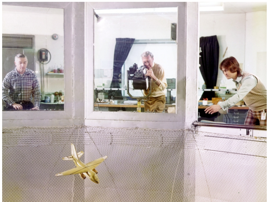
S-3 model launched into the vertically rising airstream in the Langley Spin Tunnel.
