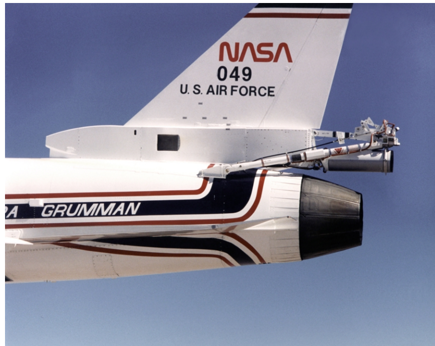
The spin parachute and truss assembly on the X-29 during high-angle-of-attack tests at Dryden.
