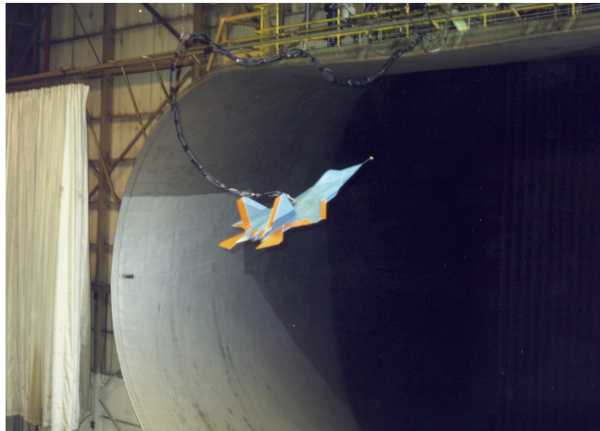
Free-flight tests of the YF-22 model in the Langley Full-Scale Tunnel in 1990.
