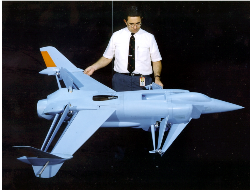
Langley researcher William Newsom with the XFV-12A free-flight model with augmentor doors on wing and canard open.
