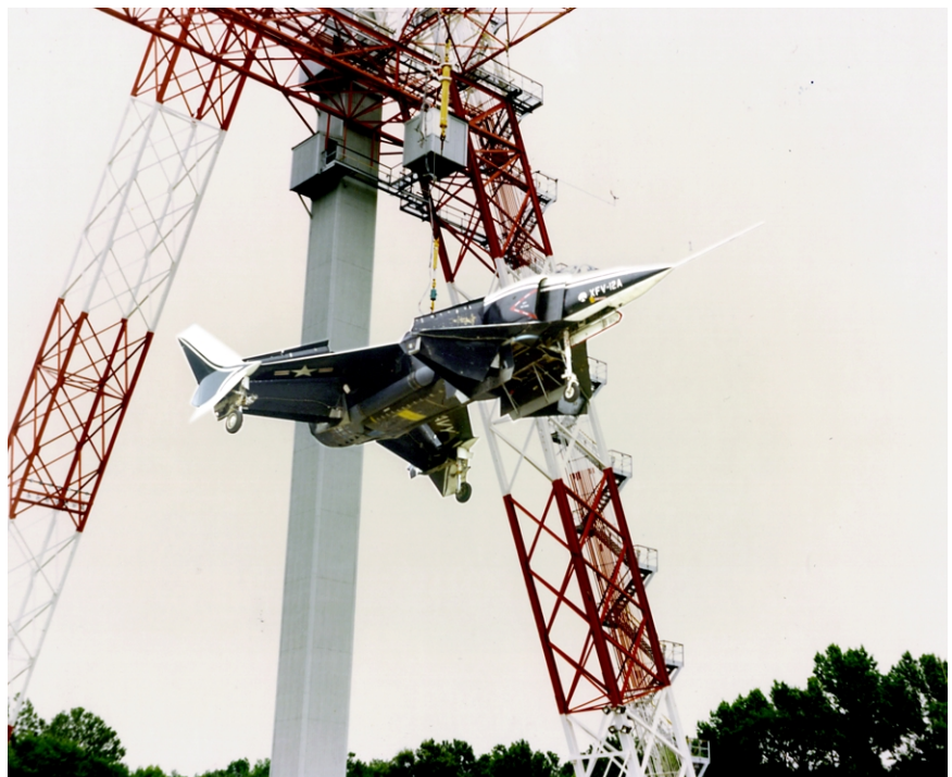
XFV-12A aircraft mounted for tethered hover flights on Langley Impact Dynamics Research Facility.
