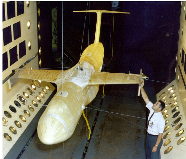
Clipped wing model of the C-5 in the Langley 16-Foot Transonic Tunnel for flutter tests.
