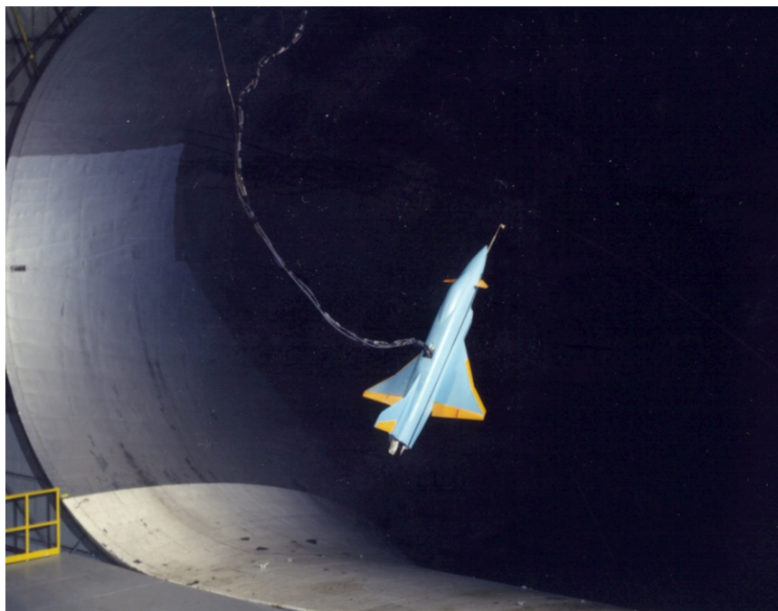
Free-flight tests of the X-31 in the Langley Full-Scale Tunnel.
