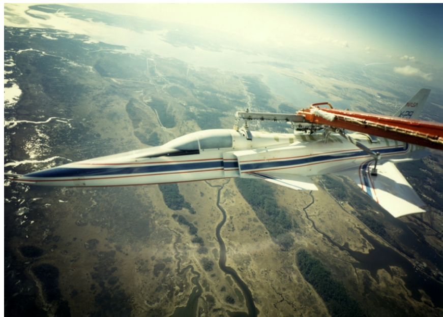
X-29 drop model mounted on launch apparatus on side of helicopter prior to release for post-stall tests.
