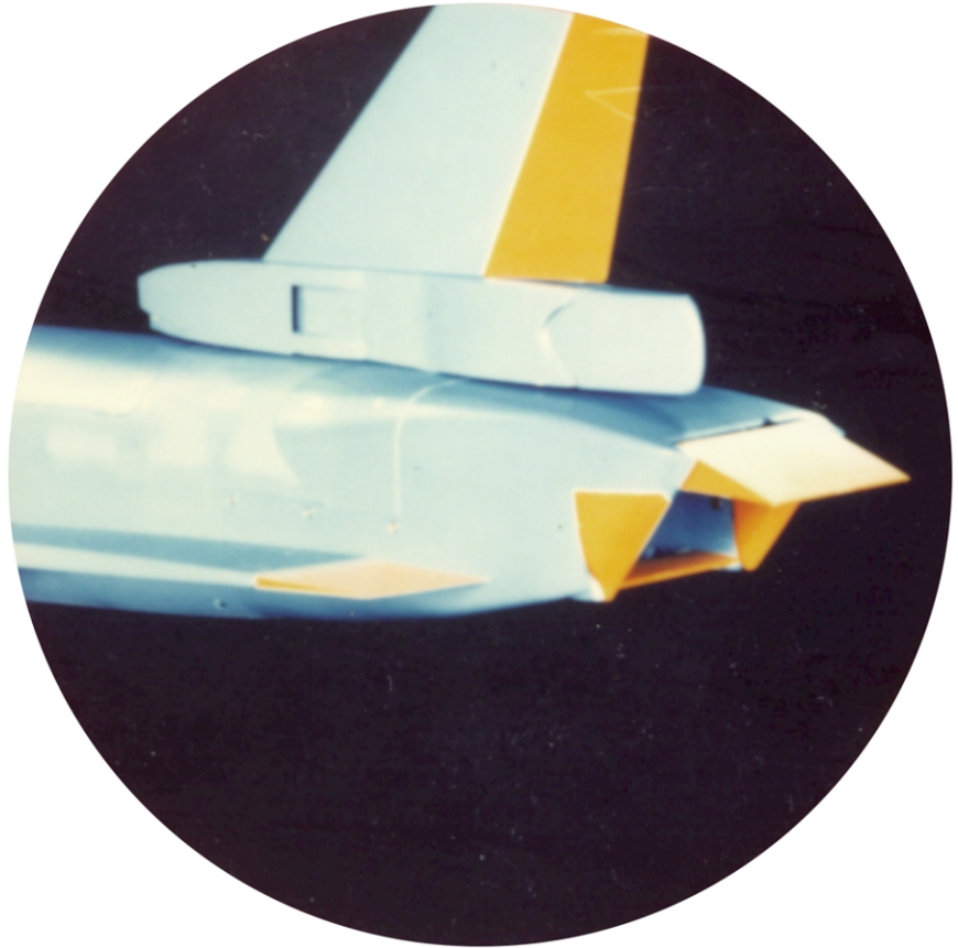
Simple ADEN-like nozzle configuration (pitch and yaw vectoring) flown on X-29 free-flight model in the Full-Scale Tunnel.
