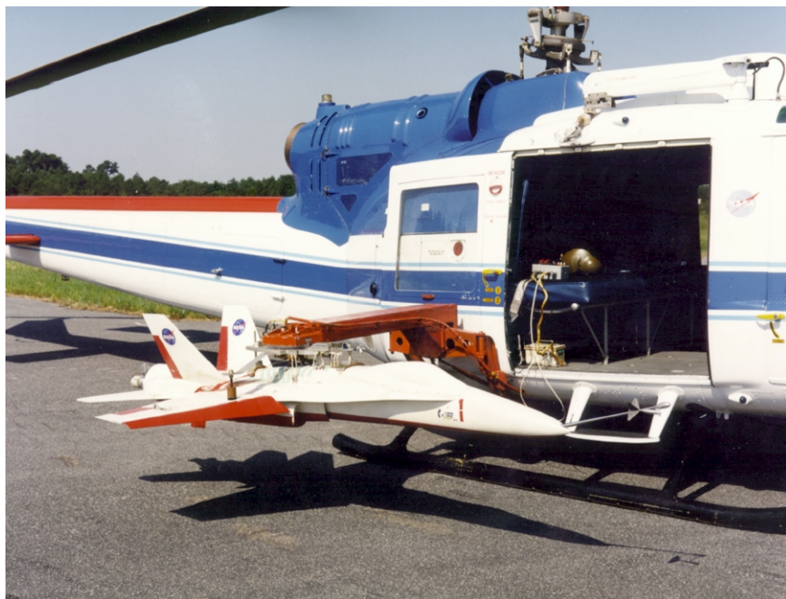
F/A-18 drop model prepared for flight in 1978.
