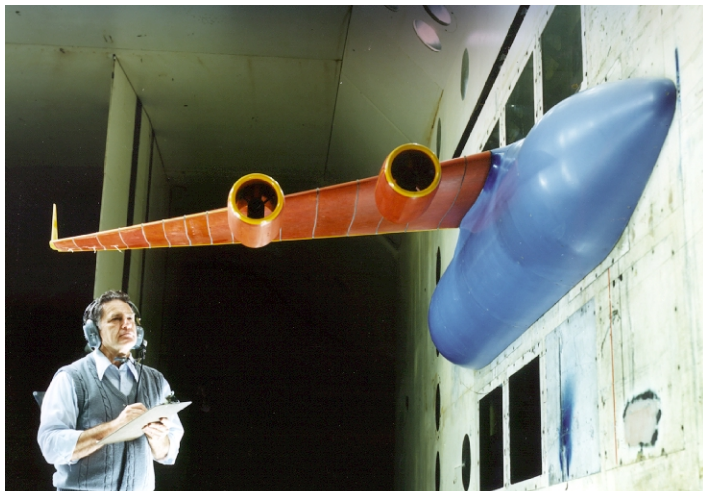
Semispan model for the C-17 wing-winglet configuration in the Langley 16-Foot Transonic Dynamics Tunnel for flutter tests.
