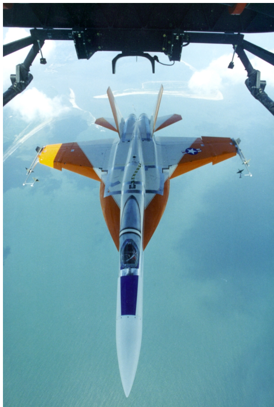
F/A-18E/F drop model immediately after release from the helicopter.
