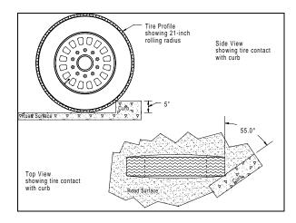
Figure 6 -- Curb and tire profiles
