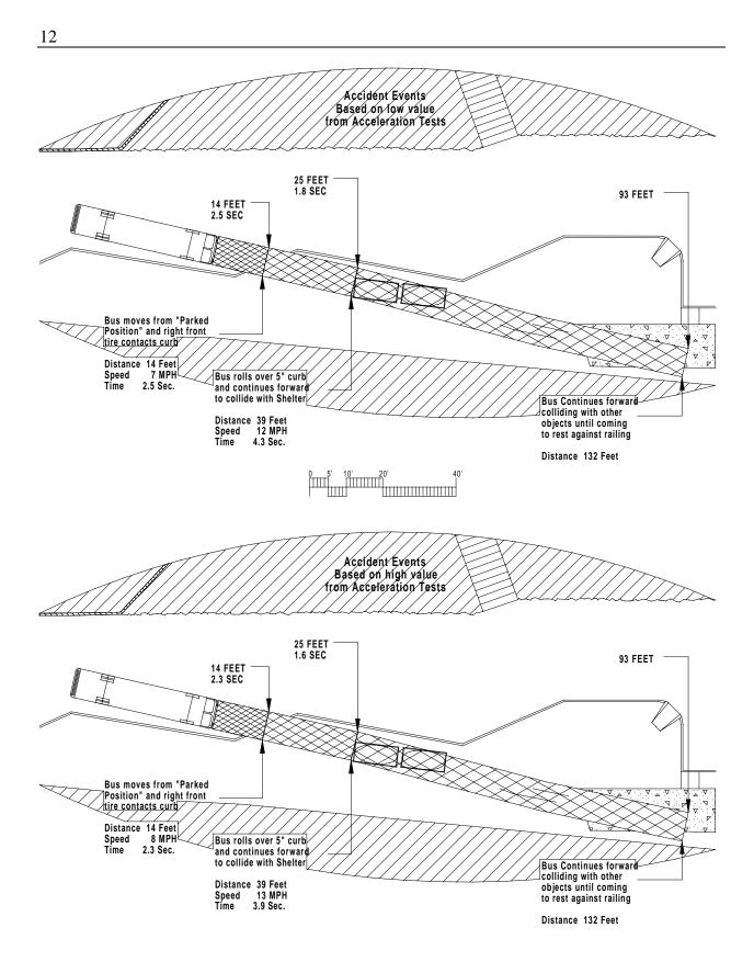
Figure 7 -- Acceleration test scenarios
