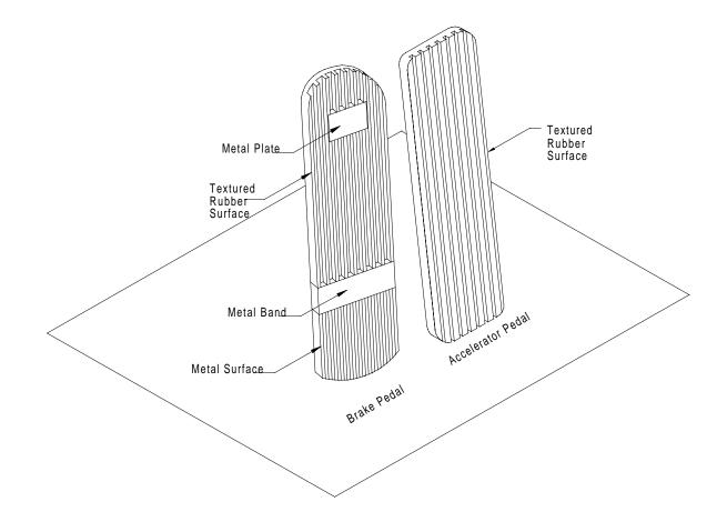
Figure 5 -- Pedal configuration
