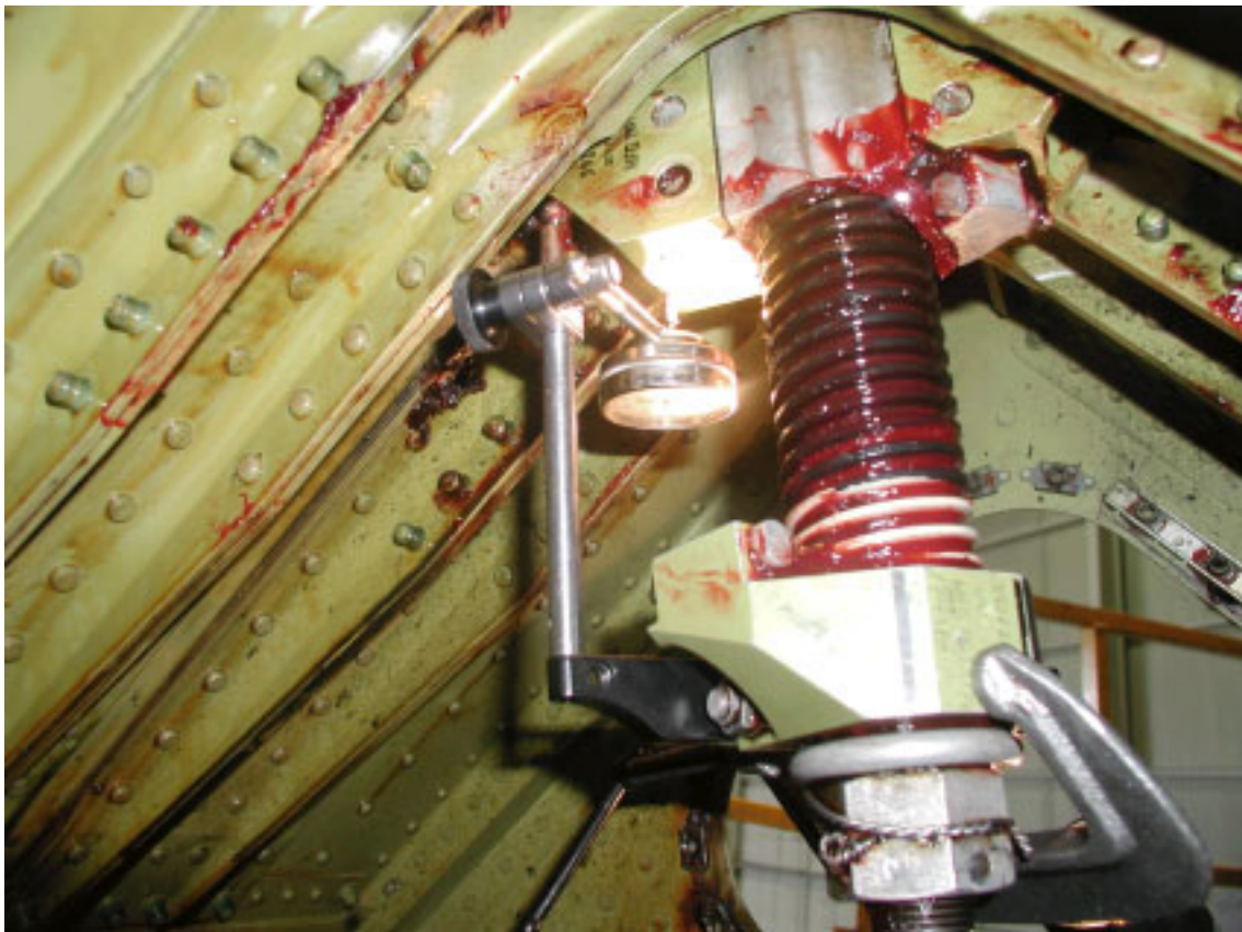
Figure 9. View of a typical dial indicator set up for end play checks.
