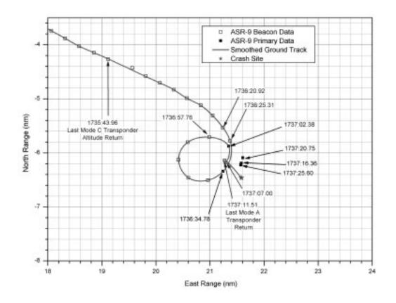
Note: Airport surveillance radar-9 (ASR-9) primary data are reflected radio signals. ASR-9 primary data returns were received until about 1737:26, about 14 seconds after the last mode A (beacon data) return. The distances shown are relative to the ASR-9 radar site at Denver International Airport.
