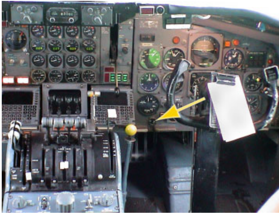
Figure 4. EPI installation on the lower left side of the first officer's instrument panel (shown by the yellow arrow), similar to that on the accident airplane.
