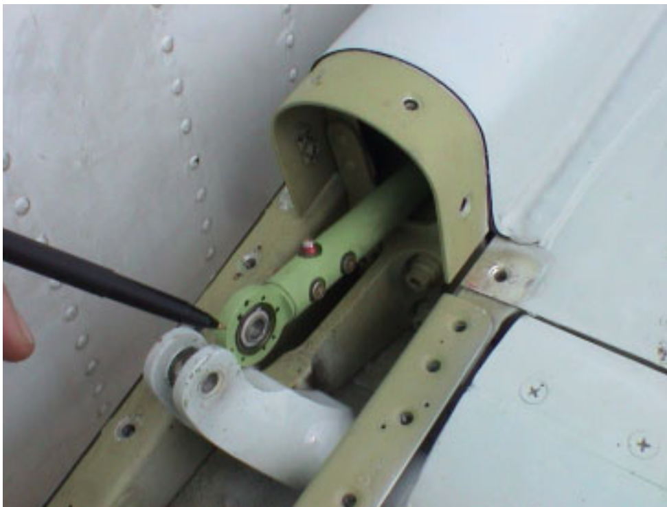
Figure 10. Photograph of the test airplane's right elevator control tab pushrod contacting the crank fitting.
