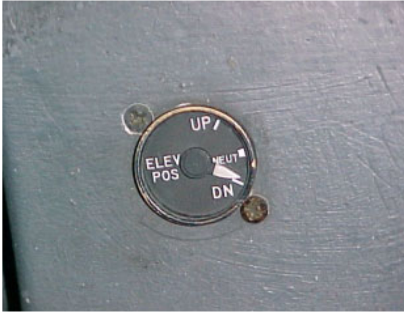
Figure 3. A photograph of an EPI gauge similar to the gauge installed on the accident airplane.
