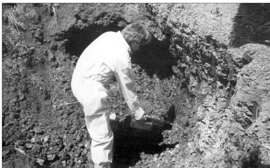
Field analyzing for volatile organic vapors with a photo ion detector (Cottonwood Field Office, Upper Columbia-Salmon Clearwater District, Idaho).
