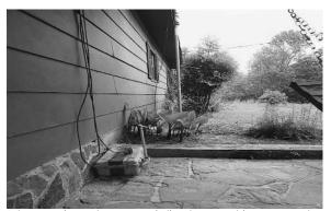
Seismograph monitors ground vibration at residence near mine operation to ensure blasting within prescribed limits.
