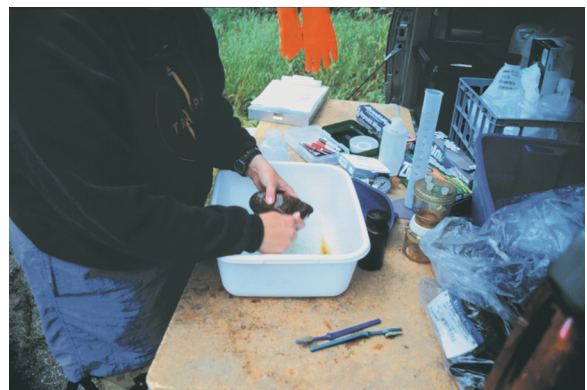
Algae samples are processed by scraping algal material from stream cobbles. Photograph by Kirby Wynn, U.S. Geological Survey.
