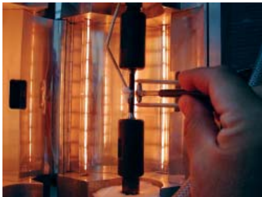
Figure 1: Instrumentation adjustment on high-temperature specimen.
