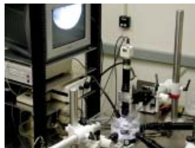
Figure 1: The computer-controlled, automated test system for measuring the biaxial mechanical properties of normo- and hypertensive pulmonary arteries.
