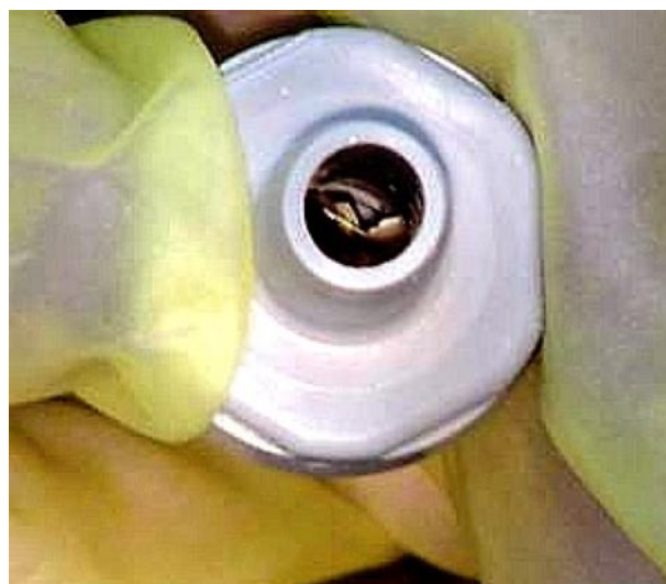
Figure 4-2. Clogged quick-disconnect fitting
