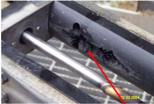
Pitting wear around the black insulators protecting the high voltage wire from the discharge
