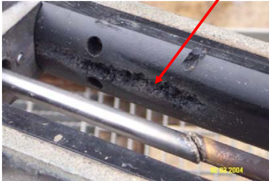
Pitting wear around the black insulators protecting the high voltage wire from the discharge
