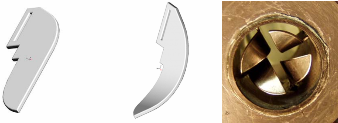
Figure 1. (a) A sketch of the SMA fin shown in its unheated, relatively soft martensite phase at a temperature below T_c . (b) The same SMA fin shown in its heated, relatively stiff austenite phase at temperatures above T_c . (c) Photo of an assembly of four such SMA fins in the new Vortigen concept.
