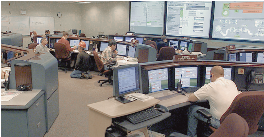
NIF’s control system handles the computerized monitoring and control of 60,000 elements throughout the system.
