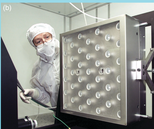
(a) A KDP crystal for NIF's optical system and (b) a deformable mirror to eliminate wavefront aberrations in the laser beam.
