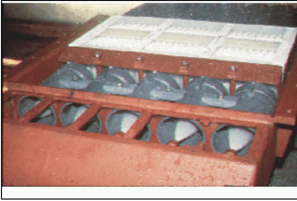
A water-powered scrubber simultaneously entrains air movement and captures dust.
