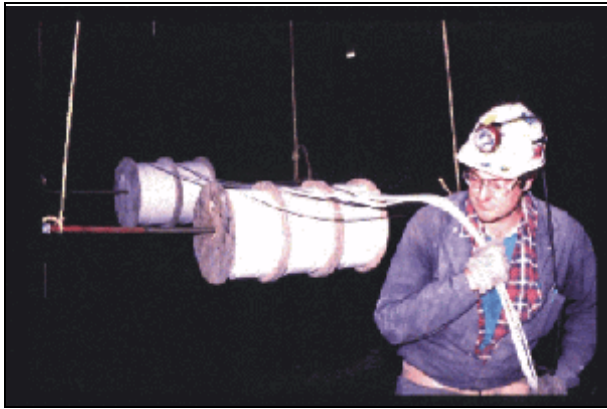
Cables connect sensitive seismometers to an underground networked data acquisition computer.
