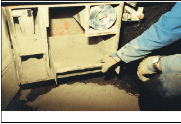
Roof bolter dust collectors require regular cleaning of the dust box and canister filter.
