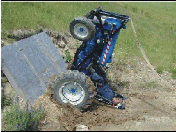
Rear upset test with mannequin.
