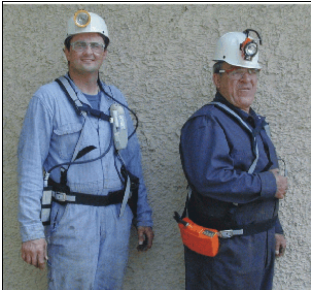
Two versions of the person-wearable dust monitor. The left contains a lapel sampler and belt pack; the right has an integrated cap lamp and dust sampler.
