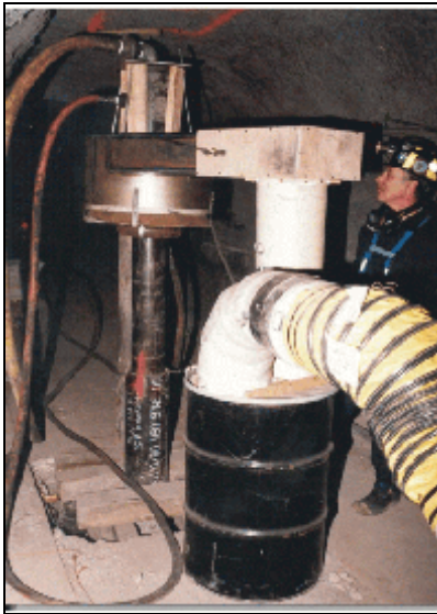
Inlet hood prototype for improved dust capture on drilling operations.
