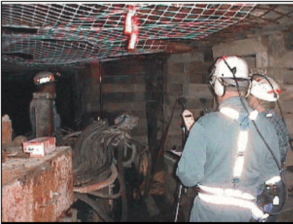
Wearing hearing protection for 85- to 90-dBA noise levels is an element of the new noise rules promulgated by MSHA.
