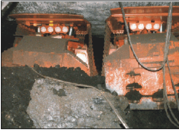
Static load/load rate monitoring system being tested on an MRS in a western U.S. coal mine.
