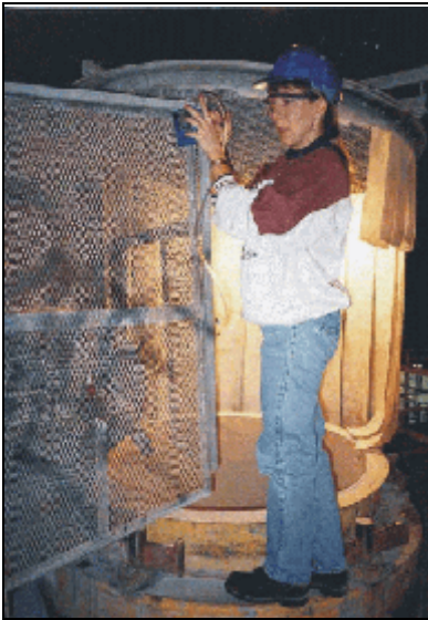
A sampling pump is being placed near the main rock crusher in a mill to collect a dust sample.
