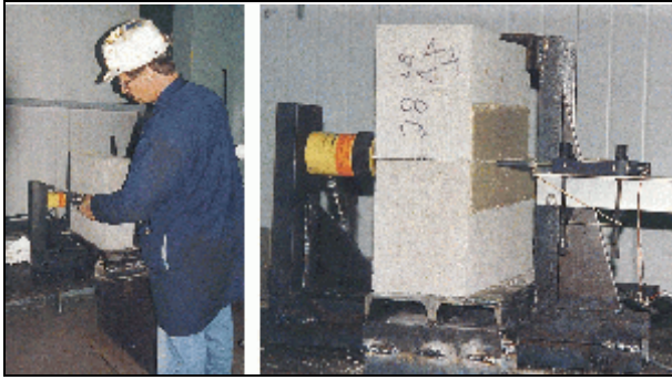
Testing of sealant strength across concrete block joint.
