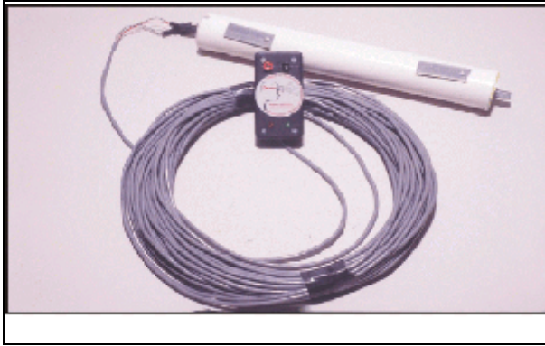
RMSS cable and read-out box.
