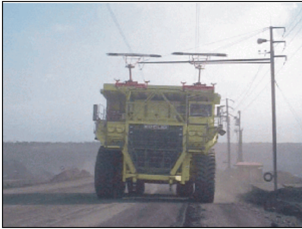
Haul trucks are expected to increase in size, and trolley power is one possibility to improve efficiency. Such innovations can impact the safety and health of mine workers. (Photo courtesy of Siemens AG.)
