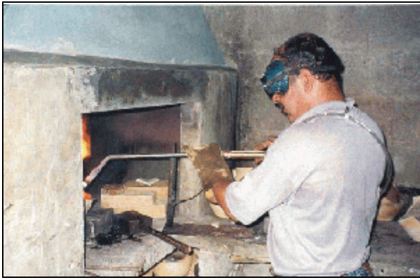
Following the processing of gold ore, a refinery worker in Bella Rica, Ecuador, burns the remaining impurities, which may include small amounts of mercury.
