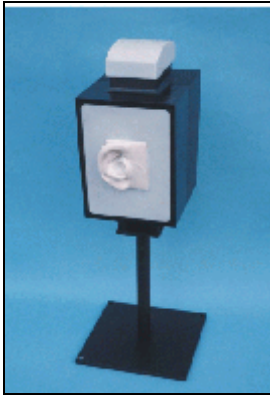
Artificial text fixture (simulated human ear) for hearing protector research.
