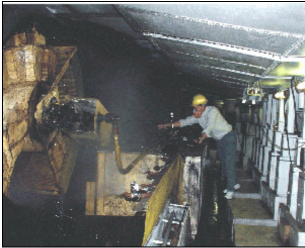
Dust sampling in a full-scale longwall gallery.
