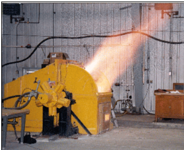
Frictional test apparatus showing ignition of methane-air.
