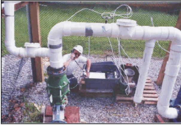
A researcher checks the cellular telephone data transmission components of the Remote Gob Gas Venthole Data Acquisition and Transmission System.
