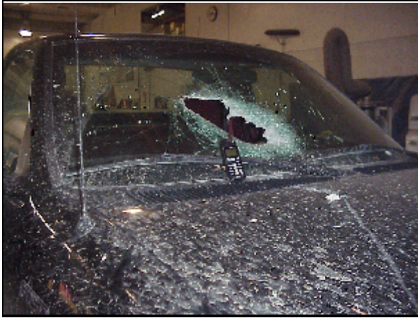
In a December 1999 accident, a baseball-sized piece of flyrock went through the window of this truck and killed the miner inside.
