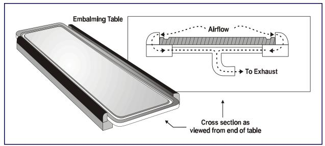
Figure 1. Diagram of Local Exhaust Ventilation Slot Hood
