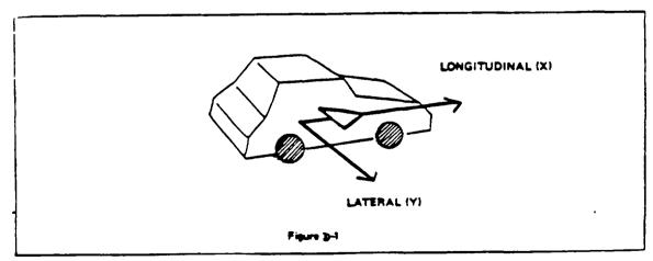
Figure D-1 shows the positive direction of the longitudinal and lateral components of Delta-V. For example, in a head-on collision, a vehicle is decelerated and the initial high positive longitudinal velocity is reduced; thus it will have a negative longitudinal De ta-V.
