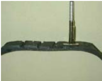
Image 1: Procedure for Tread Depth Measurement: “on the shallowest groove.”
