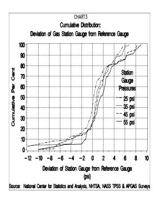
The APGAS also found that the higher the recommended tire pressure, the greater the probability of encountering a station whose gauge will over-report the actual pressure (leading motorists to under-inflate their tires). For example, at a pressure level of 25 psi, 25 percent of station gauges over-report pressure by at least 2 psi; at pressure levels of 35 and
