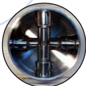
A 2-spoke superconducting resonator recently developed and tested for RIA.
