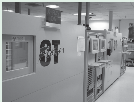
The Flash CT, built by Hytec, is a 3D tomography system used for model-based engineering and nondestructive inspection.
