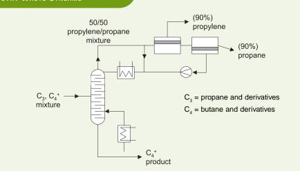
Olefin recovery from waste will use a propylene/propane membrane separation system installed on the overhead vapor from a refinery depropanizer column.
