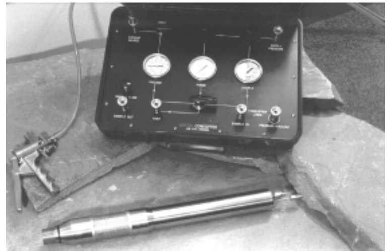
Figure 1. ConeSipper, SCAPS attachment and pneumatic valving system used to collect water and soil gas samples.
