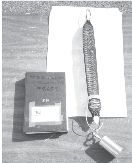
Figure 1. Typical passive diffusion bag used for groundwater sample collection (notebook shows approximate scale).
