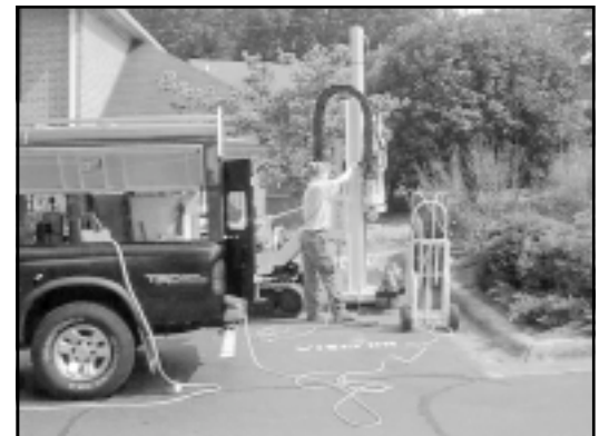
Figure 1: MIP/SC probe in operation at NSCS Athens.
