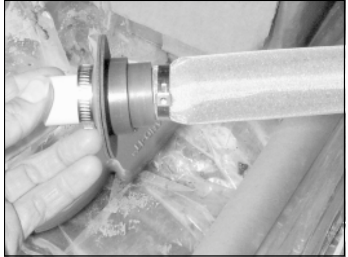
Figure 1: Preparation of a 3/4-inch prepack direct-push well. The stainless steel enmeshed sand pack sleeve (manufactured by GeoInsight) covers the slotted portion of the PVC riser pipe. The flanged area protects the screen from backfill materials.
